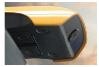
**Advanced Around View Monitoring** (AAVM) and Intelligent Moving Object Detection (IMOD) The optional Advanced Around View Monitoring (AAVM) system gives you a 360° overview of your immediate working environment. It also includes Intelligent Moving Object Detection (IMOD) technology that senses and warns you when people or objects come within five metres of the machine.
