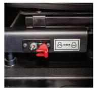
**Emergency stop switch** The engine can be shut down immediately using an emergency stop switch located at the base of the seat.
