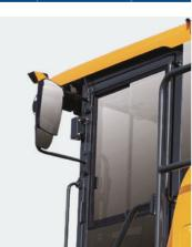
Foldable side mirror The side mirror is easy to adjust for optimal visibility and can be folded away to prevent damage during transportation.
