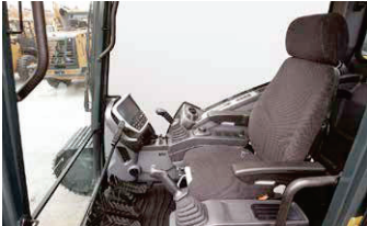
Air suspension seat and ergonomic joysticks The HX380AL has a luxurious air suspension seat with heating as standard. The ergonomic joysticks make operation comfortable and intuitive.
