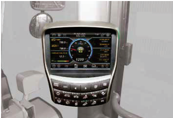
Wide touchscreen monitor The HX380AL features an 8-inch display with a touchscreen and excellent legibility. It allows quick and easy access to machine status information at any time during operation.
