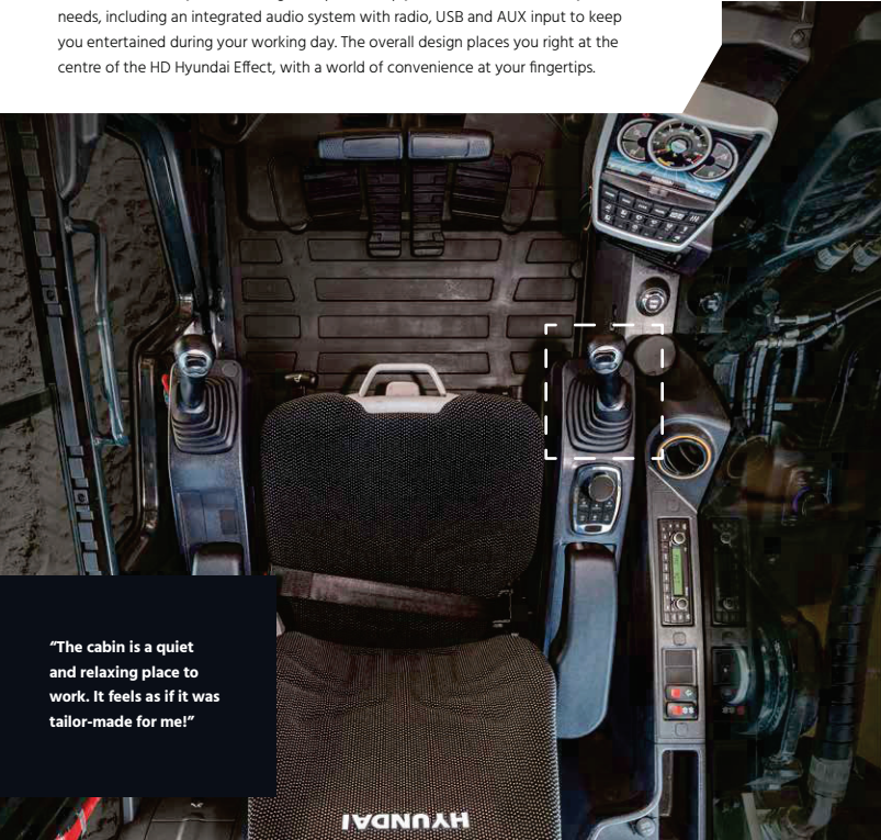
Proportional auxiliary hydraulic controls (option) Sensitive regulated proportional controls are available as an option. They enhance work results by enabling smooth and precise operation of hydraulic attachments via the joysticks.
