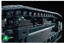
The larger rollers in the newly upgraded undercarriage account for superior performance and longevity.
