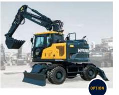
Floating boom function The floating boom setting allows the boom to move up and down freely under its own weight. This enables effortless levelling of surfaces.
