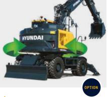
Fine swing control Fine swing control enables smooth movement at the beginning and end of swing operations. This improves precision in a wide range of applications and reduces spillage from the bucket.
