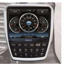
Wide touchscreen monitor The 8-inch touchscreen is one of the largest on the market and features WiFi connectivity, allowing operators to take advantage of smart technologies as they work.
