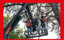
Basket 2.10 m - Side door Manitou has wider baskets with a side door for easy access.
