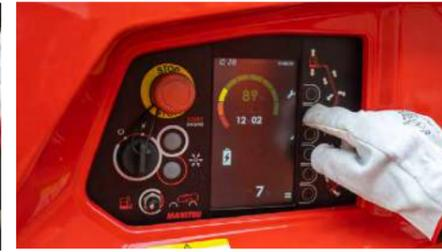
The large screen at the lower control box offers additional information to the top control box for operator and allows technicians to carry out a quick diagnosis, consult the machine memory and many other functions.
