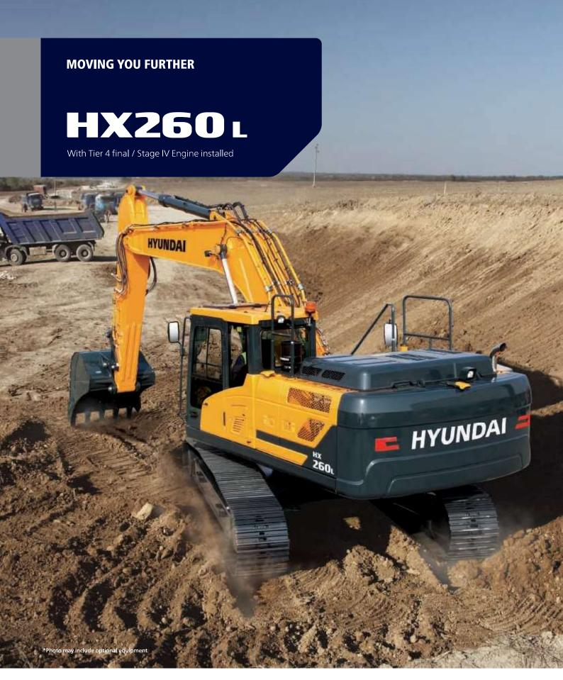
**Net Power** SAE J1349 / 133 kW (179 HP) at 1,950 rpm **Gross Power**
