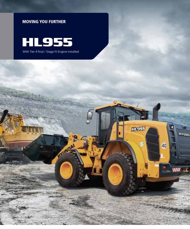
**Net Power** 147 kW (197 HP) / 2,200 rpm **Gross Power** 149 kW (200 HP) / 2,200 rpm **Travel Speed** 38.5 km/h (23.9 mph)
